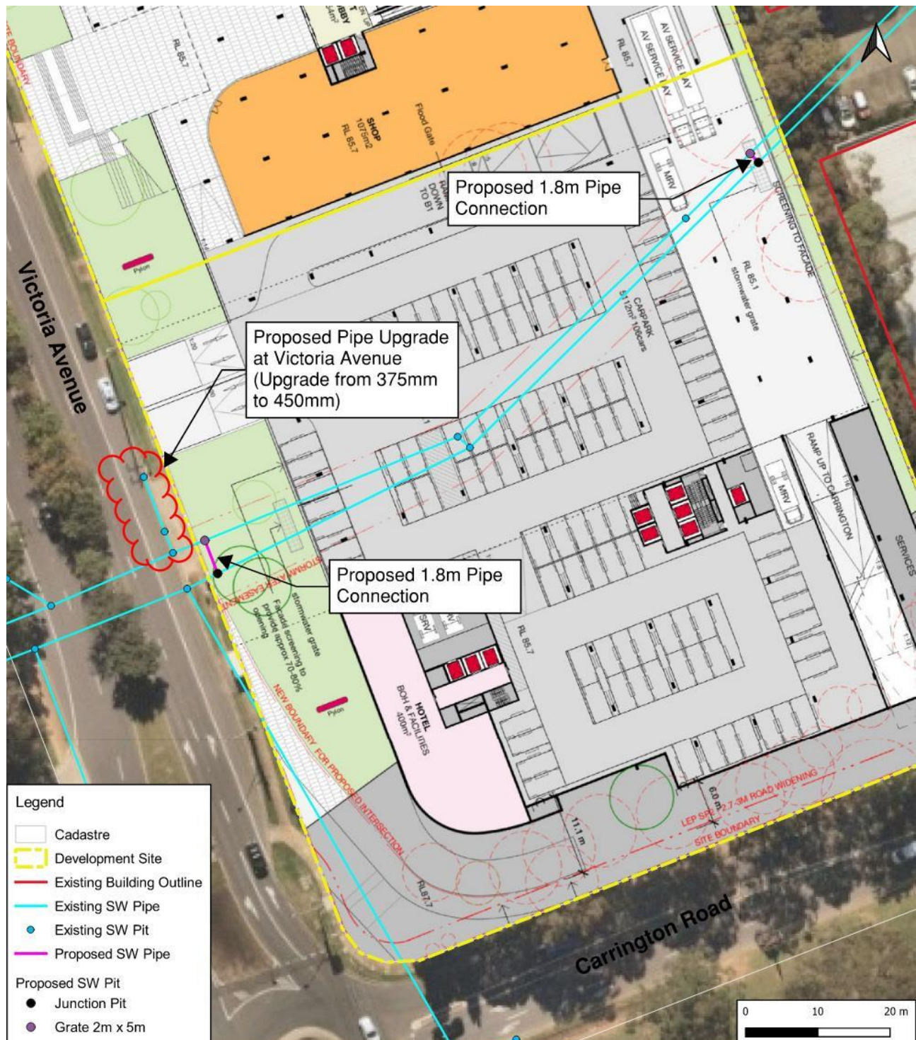
Figure 20 – Proposed Pipe upgrade at Victoria Avenue
